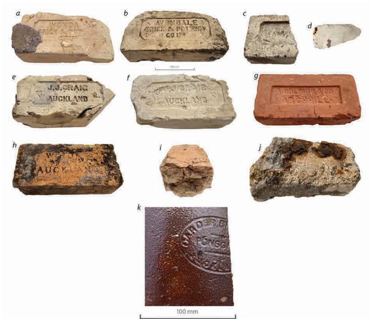
Figure 25. Bricks and Pipe from Carrington Early Works. a-b, AVONDALE BRICK AND POTTERY CO LTD brick; c, CARDER BROTHERS brick; d, unidentified white brick; e, J.J. CRAIG AUCKLAND brick with moulded 45° point; f, J.J. CRAIG AUCKLAND; g, A. DOLPHIN & CO ARCHHILL brick; h, W. HUNT AUCKLAND brick; brick cross section showing poor mixing of clay; j, brick showing poor cohesion of clay matrix; k, CARDER BROTHERS PONSONBY AUCKLAND glazed pipe.
